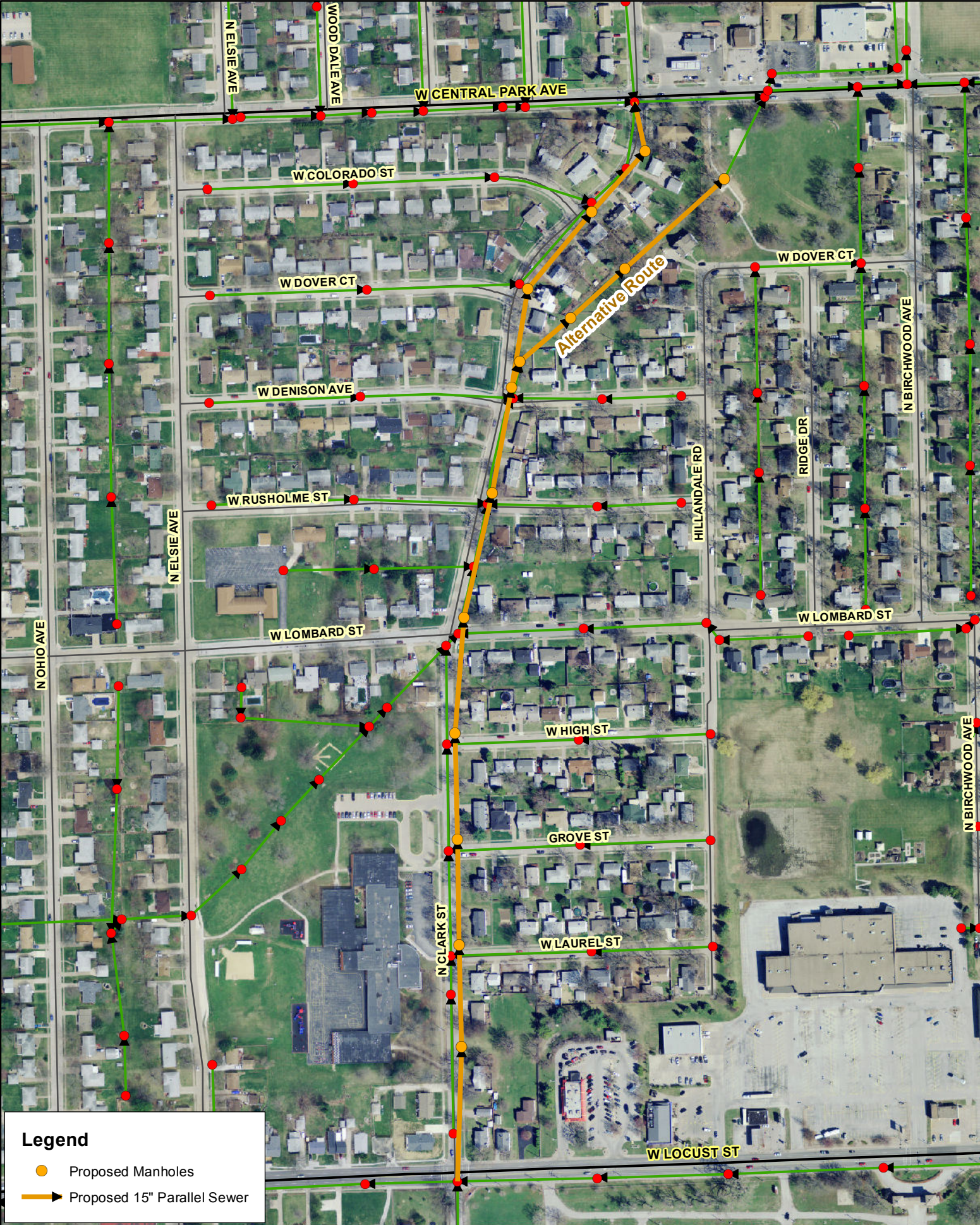
Birchwood Area Parallel Sanitary Sewer
