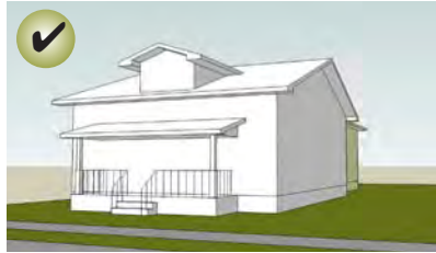
One story attached addition
