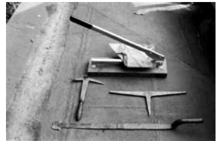
These traditional slater's tools are used to cut and trim, hammer, measure, and rip out nails. Photo: Jeffrey S. Levine.
