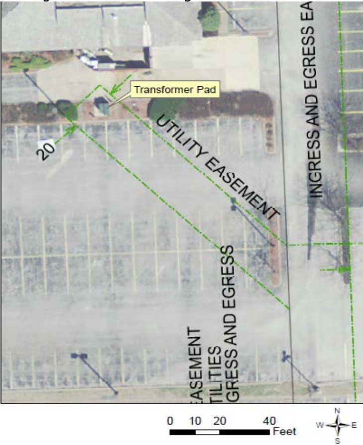
Existing easement on existing site
