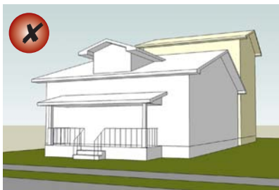
Two-and-a-half story addition with connector Addition is set back behind the original and accessed by a connector.
