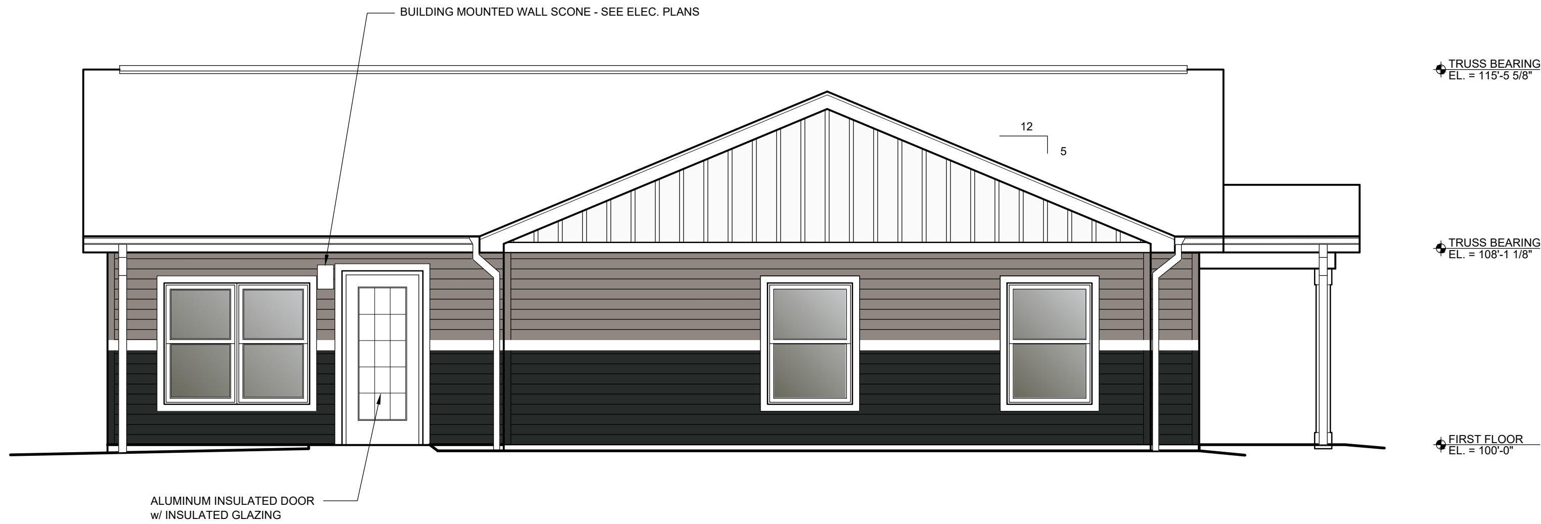
BUILDING #3 ELEVATION CLUBHOUSE SCALE: 1/4" = 1'-0"
